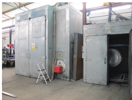
Polymerization ovens, 3x3x5 meters
