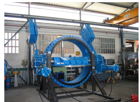
Overspeed valve DN2000 PN25, double arm
