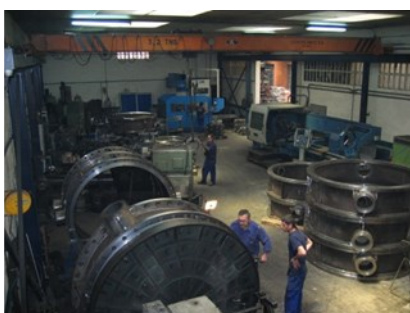
Interior plant view – big diameter valves
