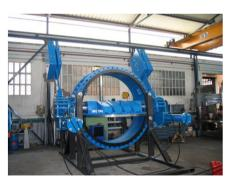
Overspeed valve DN2000 PN25, double arm
